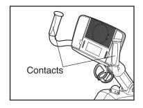
heart rate, hold the handgrip pulse sensor, with your palms resting against the metal contacts. **Avoid moving your hands or gripping the contacts tightly.**
